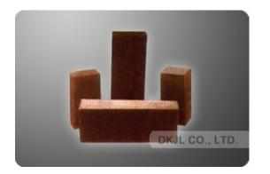
Our company can supply not only conventional magnesia bricks, but also high purity magnesia bricks and electrofused magnesia bricks. This kind of products are manufactured with high purity magnesia clinker and electrofused magnesia as raw material that contains MgO from 96% to 98%,by high pressure moulding and high temperature burning.
