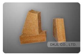
Clay bricks use Chamotte that the fire clay is calcinated as the main material. These bricks consist of fire clay and binder. The chemical components of these bricks are SiO2 and Al2O3. (Al2O3=25~40%) fireclay bricks are cheap so that they are used for all kinds of industrial furnaces. The main applications are the low temperature parts such as blast furnaces and hot blast furnaces,
